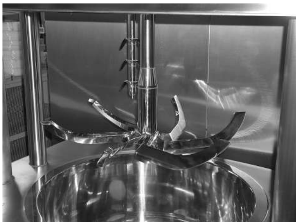
Figure 8 Example of a special pelletizing mixer arm. (Courtesy of Collette NV, Belgium.)
