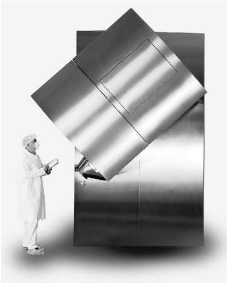
Figure 1 UltimaPro™ 600 microwave/vacuum single-pot processor with swinging bowl. (Courtesy of Collette NV, Belgium.)
