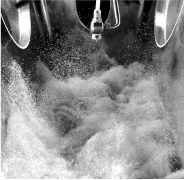
Figure 5 Continuous fluid bed processor during operation. (Courtesy of Heinen Trocknungstechnologie GmbH, Varel, Germany.)
