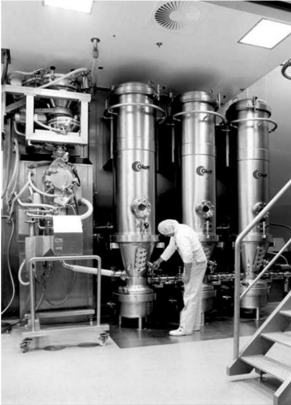
Figure 7 Multicell semicontinuous granulation processor. The dosing processor and granulation unit can be seen on the left side. (Courtesy of Glatt GmbH, Binzen, Germany.)
