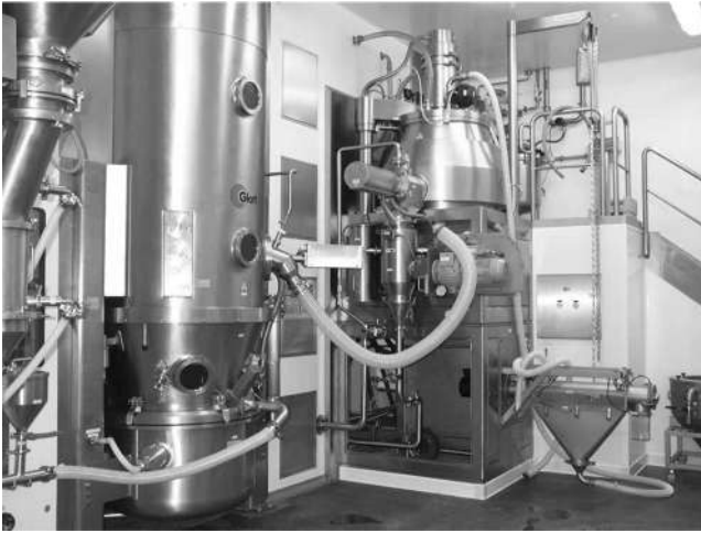
Figure 35 Loading of fluid bed from high-shear mixer. (Courtesy of the Glatt Group.)
