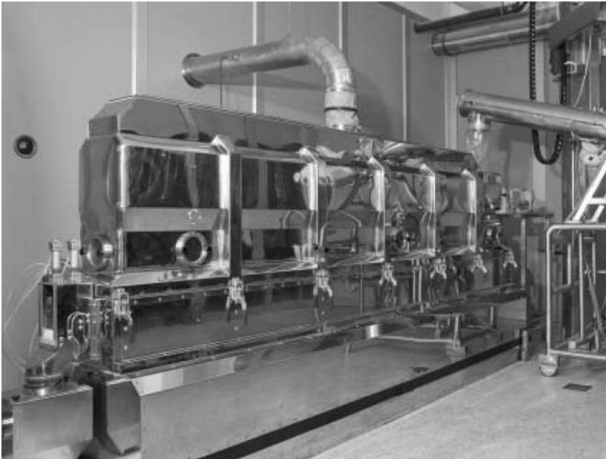
Figure 4 Heinen continuous fluid bed processor. (Courtesy of Heinen Trocknungstechnologie GmbH, Varel, Germany.)
