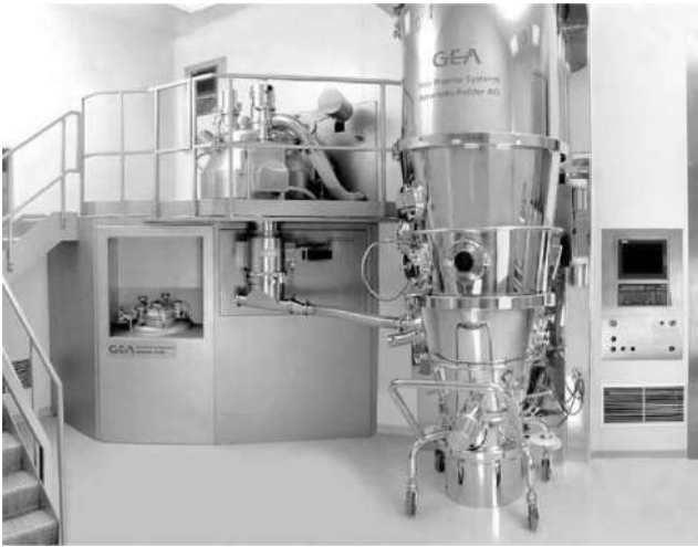
Figure 4 An integrated pharmaceutical manufacturing facility (high-shear granulator–conical screening mill–fluid bed drier).
