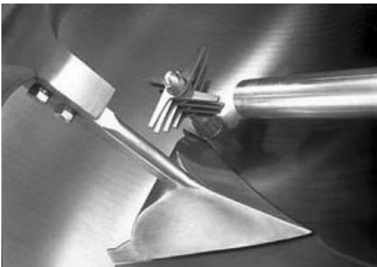
Figure 8 Photograph of a plough-shaped mixing blade and a chopper inside a horizontal high shear mixer granulator. (Courtesy of Loedige.)
